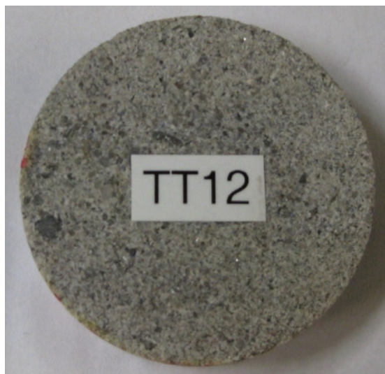
Figure 12 Biscuit shaped piece of core for transverse tensile test
