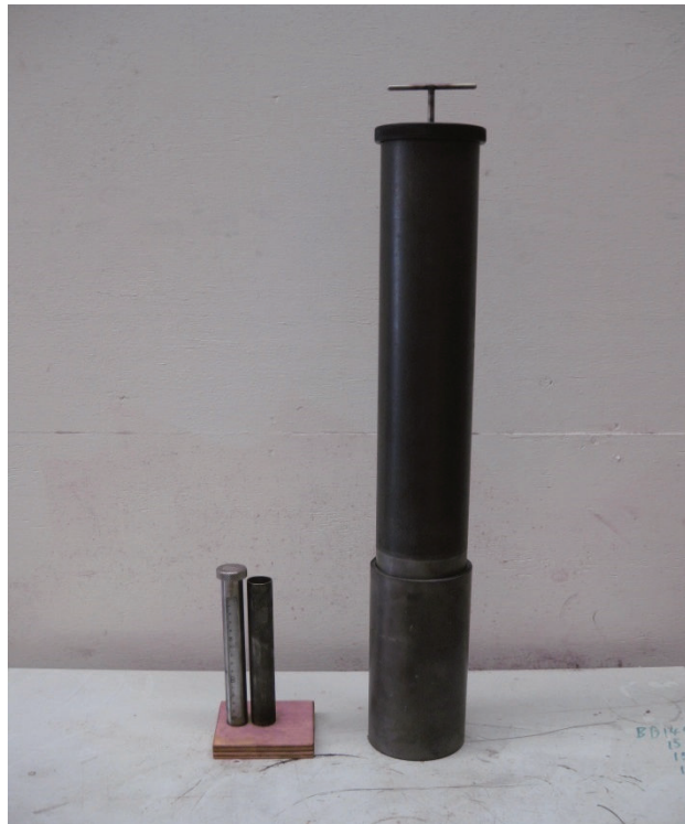
Figure 18 Protodyakanov drop hammer apparatus (right) and measuring cylinder (left)
